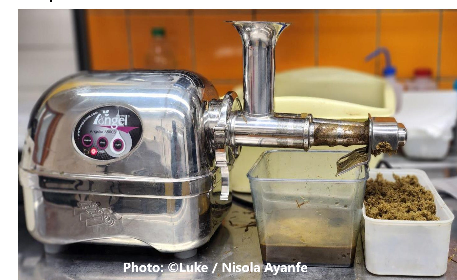
Figure 2. Mechanical pressing of a) fresh grass using a pilot scale single screw press, b) ensiled biomass using a lab-scale double screw press.
