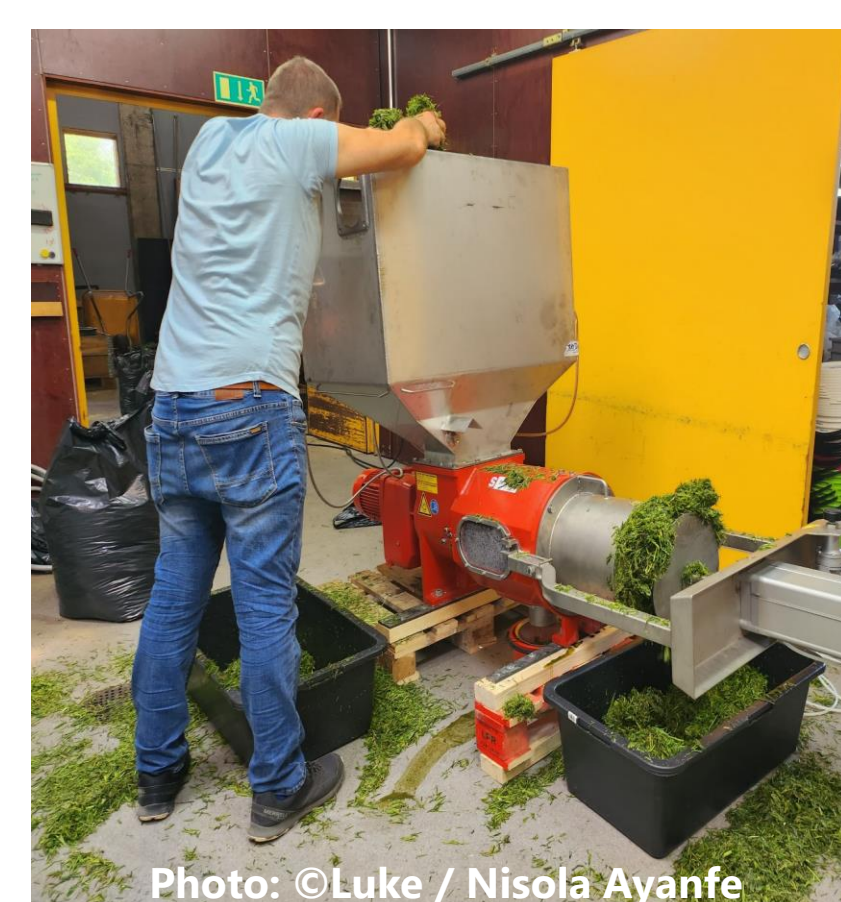
Figure 2. Mechanical pressing of a) fresh grass using a pilot scale single screw press, b) ensiled biomass using a lab-scale double screw press.
